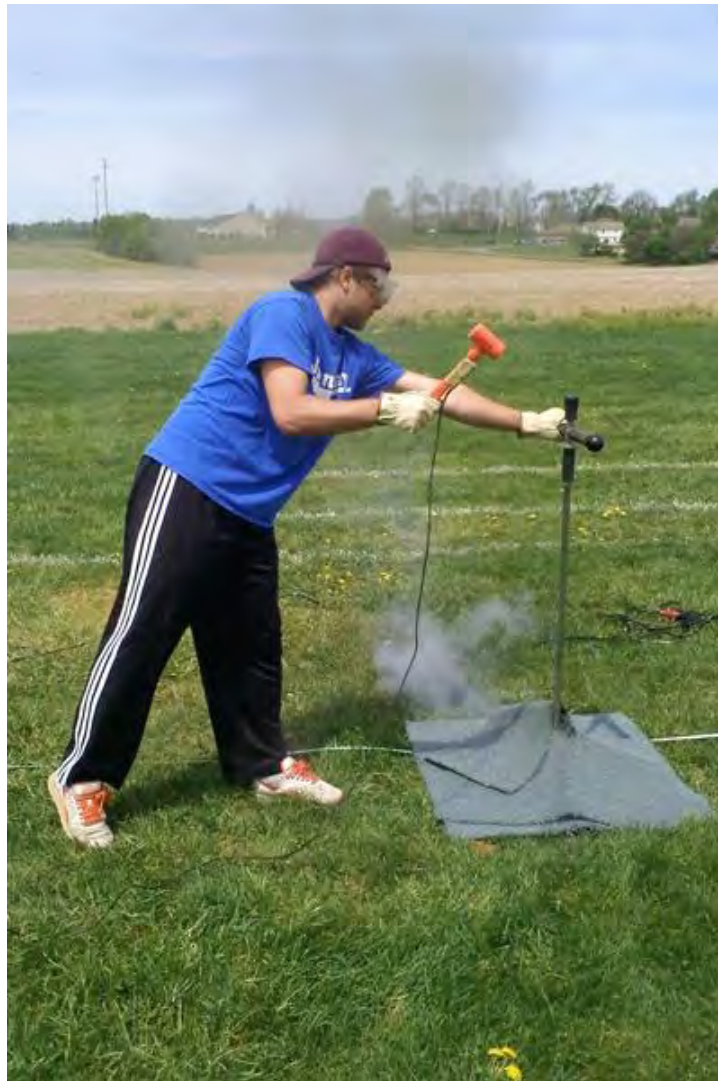
Betsy seisgun (1) with plastic splatter guard, shell holder(2), hammer(3) and shells of various sizes
